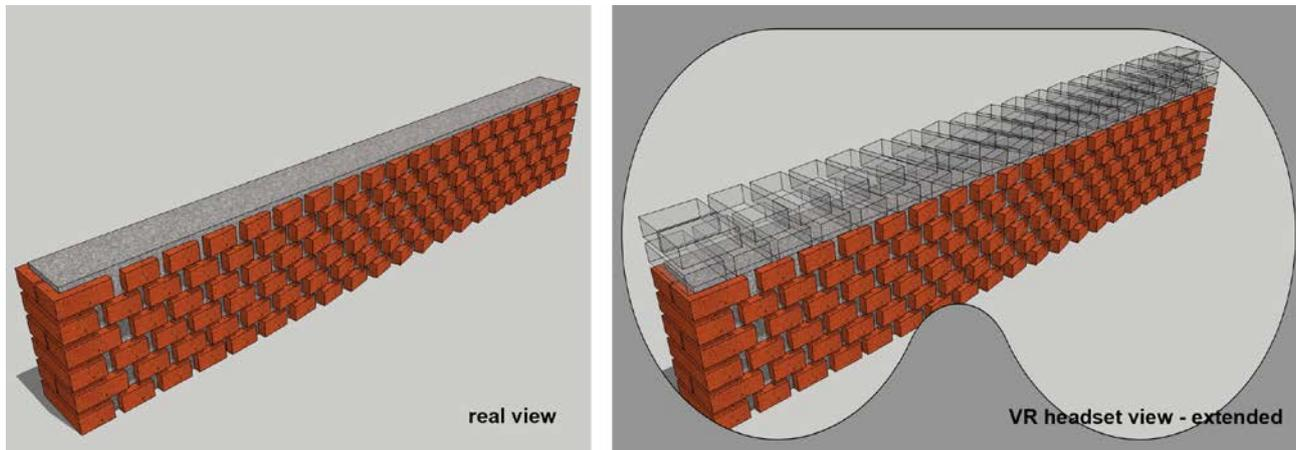
Figure 4: General scheme of working on parametric model with VR headset on a building site - displaying next elements positions in extended reality (Author's materials).
