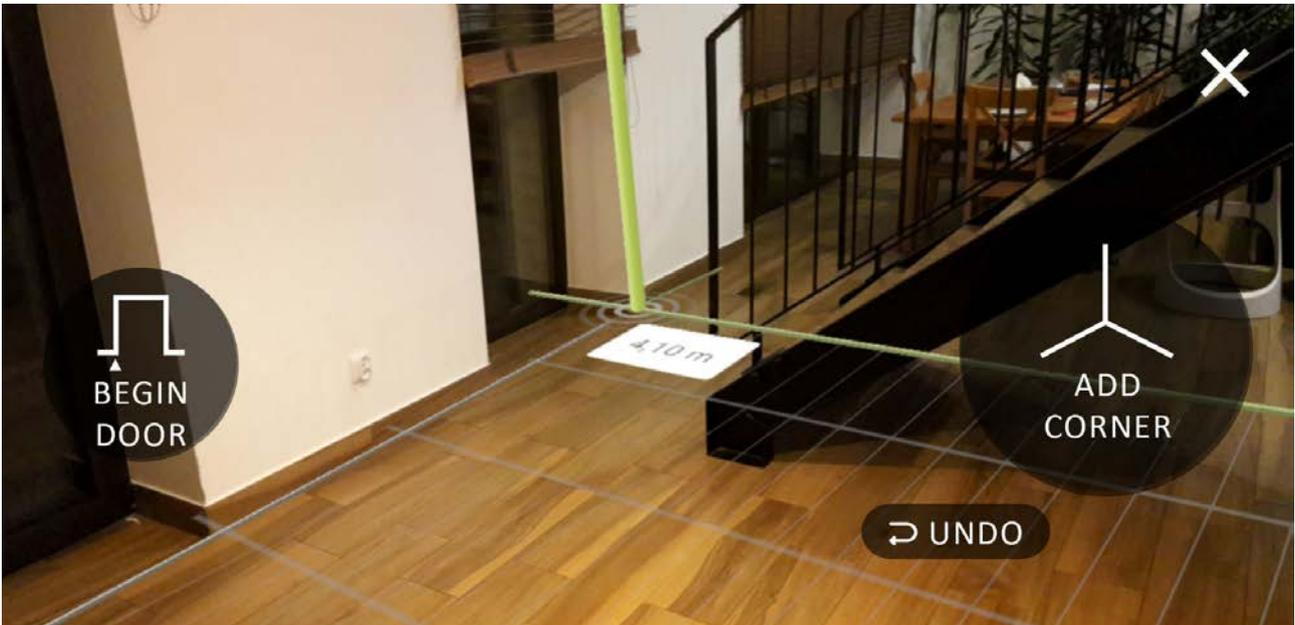
Figure 3: Example of the *magicplan* app screen. After calibration a starting point is set on one corner of a room; then real time measurements are available. Locking the positions of all edges will lead to a compact plan of the room (Author's material).
