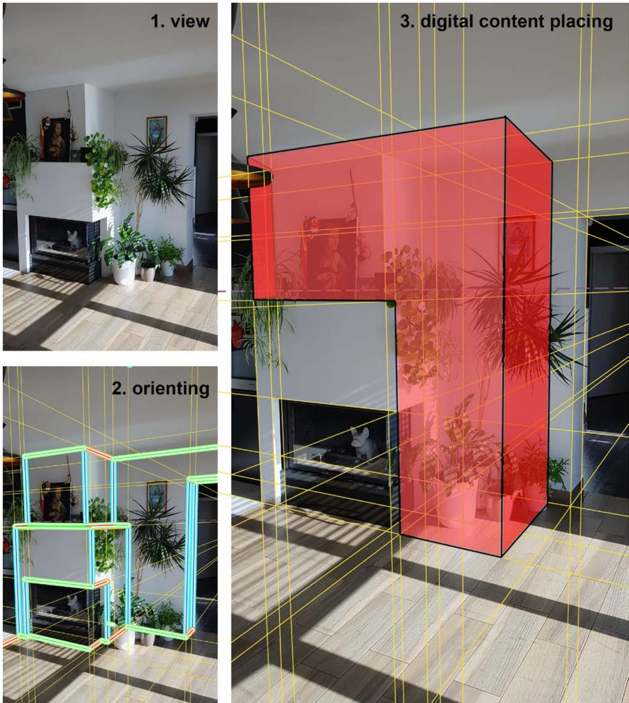
Figure 2: Augmented reality in use - 1) view capture; 2) description of coordinates and orientation; and 3) placing oriented digital 3D content - endless loop for real time effect (Author's materials).
